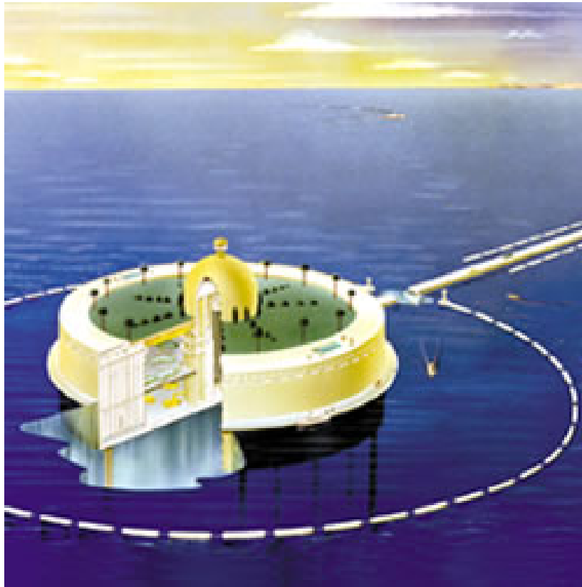
Figure 21. Nuplex Island consisting of nuclear power plants supplying fresh water and electricity for an Agro Industrial complex. Source: ORNL.
