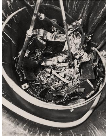
Figure 62. Damaged core resulting from steam explosion caused by a criticality accident in the military Small Low power reactor experiment SL-1 BWR. A worker inadvertently yanked out a control rod beyond the set limit during a maintenance procedure. The core became supercritical, boiled off the steam causing a steam explosion. The drying of the moderator stopped the fission reaction, even though the decay heat generation would have persisted for a while.
