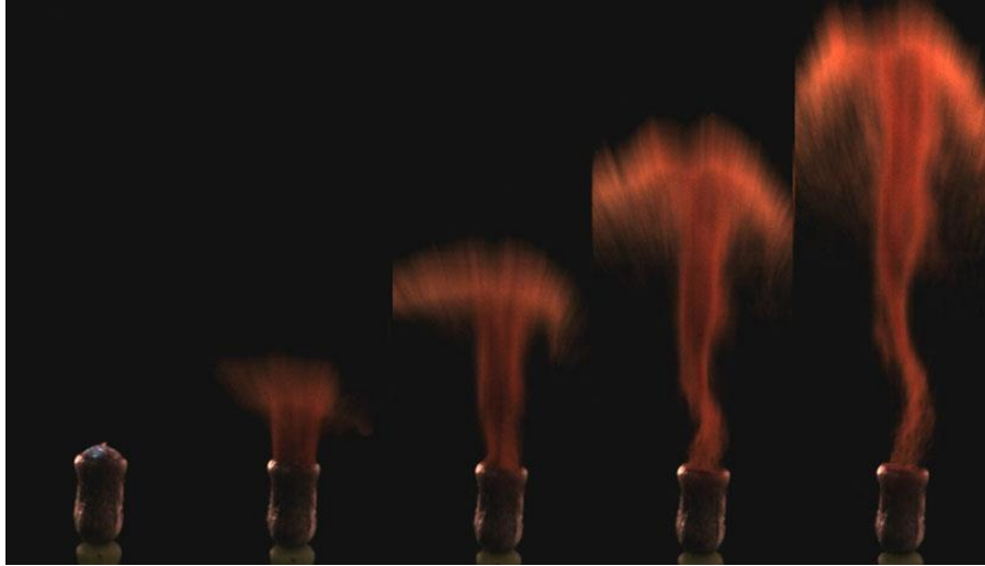
Figure 60. Exploding vortices suggest a steam explosion occurrence at unit 3.
