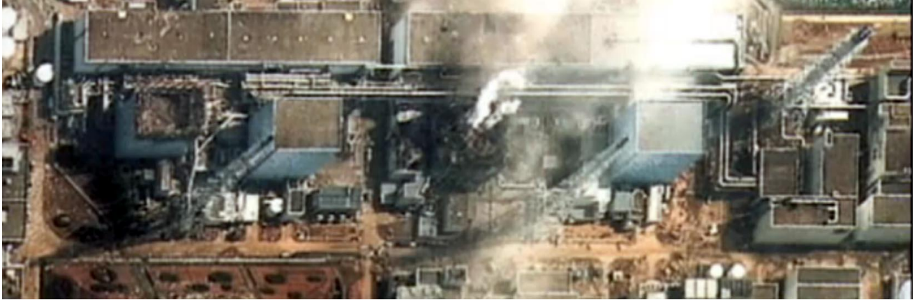
Figure 30. Remnants of a hydrogen explosion in Fukushima unit 1 (far left) exposing reactor loading deck and burying it under concrete rubble. Fire and a hydrogen explosion associated with steam depressurization and fuel damage occurred in unit 3. Fire starting at side of building in unit 4 may have originated from hydrogen generated in unit 3 that was piped into the shut-down unit 4, on March 15, 2011. Photo: DigitalGlobe.
