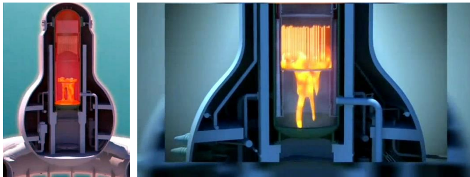
Figure 42. Core meltdown modelling of unit 1.
