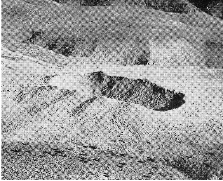
Figure 62. Multiple five-row 1.1 kT TNT charges Buggy channel cutting experiment in basalt hard rock. Source: LLNL.
