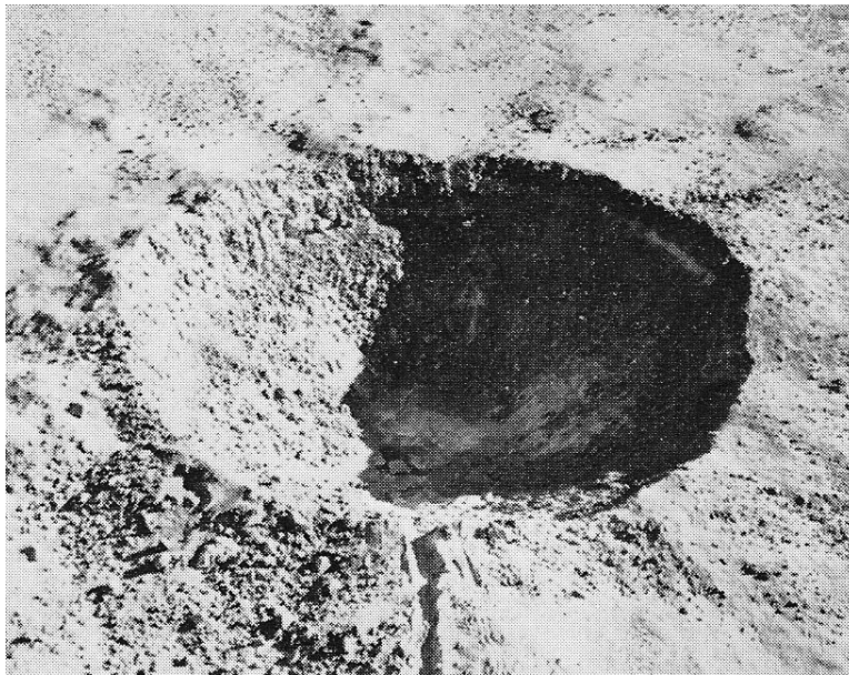
Figure 59. Single cratering 35 kT TNT charge in basalt hard rock, Schooner experiment. Source: LLNL.
