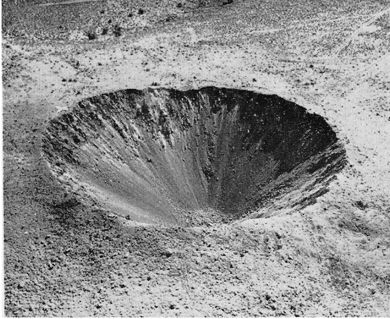
Figure 60. Cabriolet 2.3 kT TNT single shot experiment in basalt. Source: LLNL.
