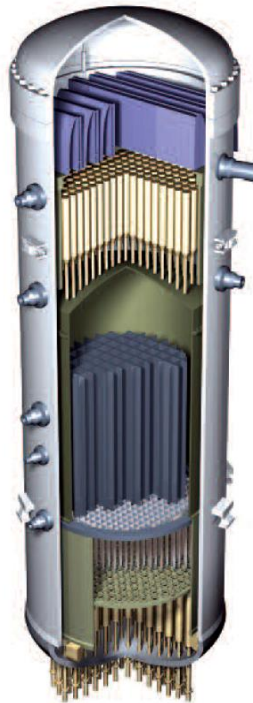
Figure 27. ESBWR pressure vessel. Natural circulation is established because of density differences between water in the vessel annulus and the steam/water mixture inside the shroud
