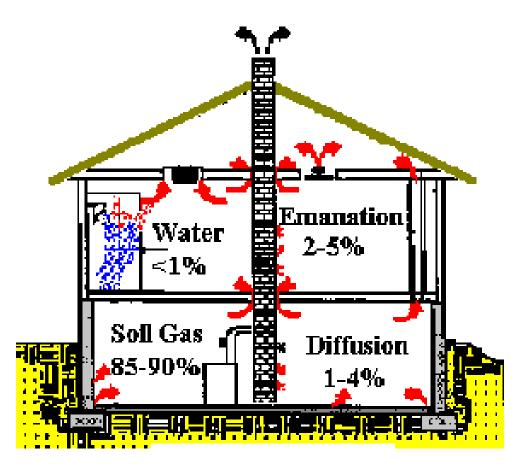
Fig. 6: Source of radon gas into a typical residence.
