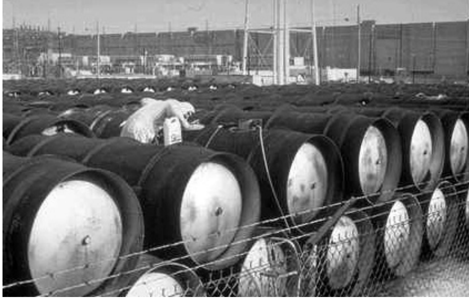
Figure 26. Uranium hexafluoride UF_6 storage cylinders.
