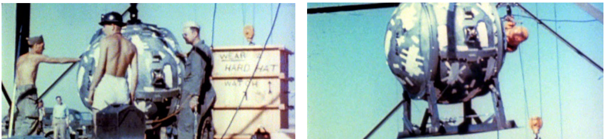
Figure 33. Trinity device before installation of initiators.
