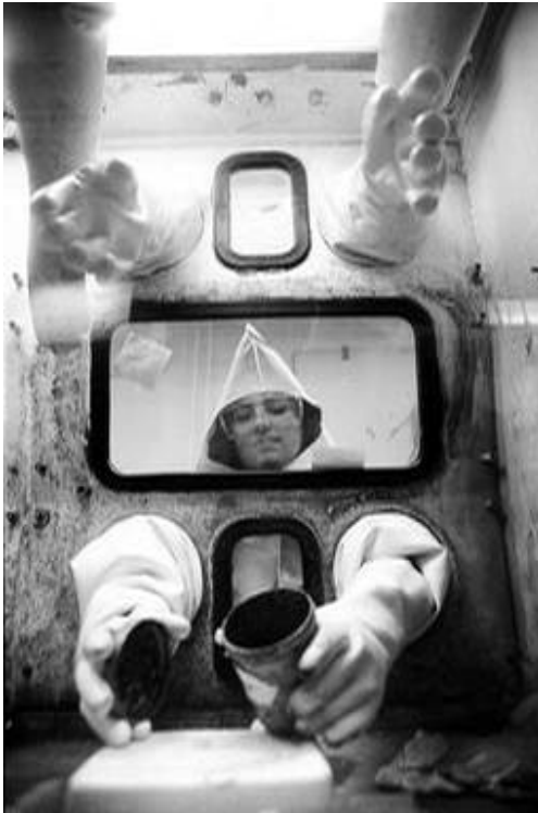
Figure 28. Inert gas plutonium glove box.
