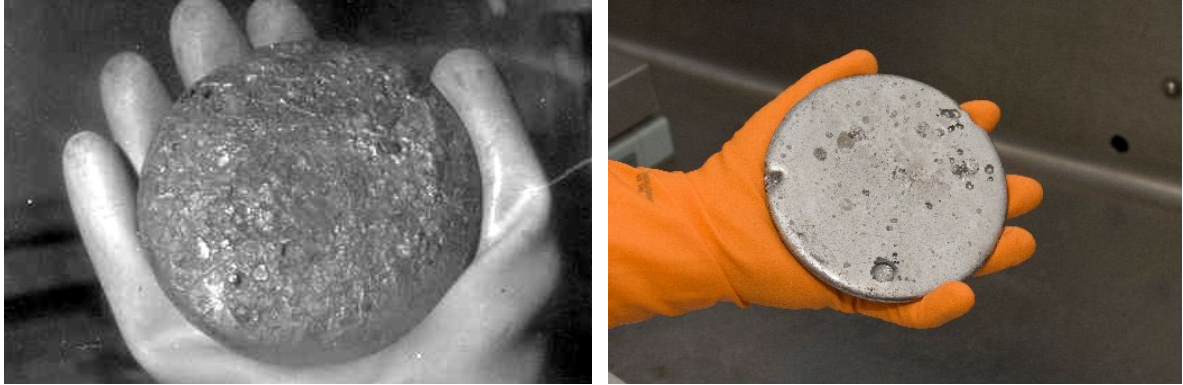
Figure 29. Finished plutonium puck or button (left) and enriched uranium ingot (right).
