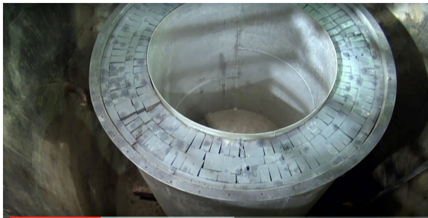
Figure 4. Graphite blocks reflector surrounding an unfinished reactor core.
