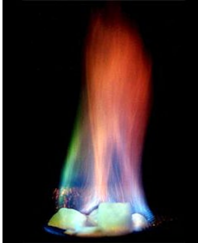
Figure 100. Clathrates or methane hydrates from the bottom of the oceans. The methane will ignite in ice form, hence the "fire ice" moniker. Source: USGS.
