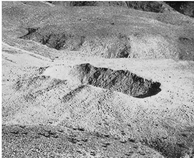
Figure 80. Multiple five-row 1.1 kT TNT charges Buggy channel cutting experiment in basalt hard rock. Source: LLNL.
