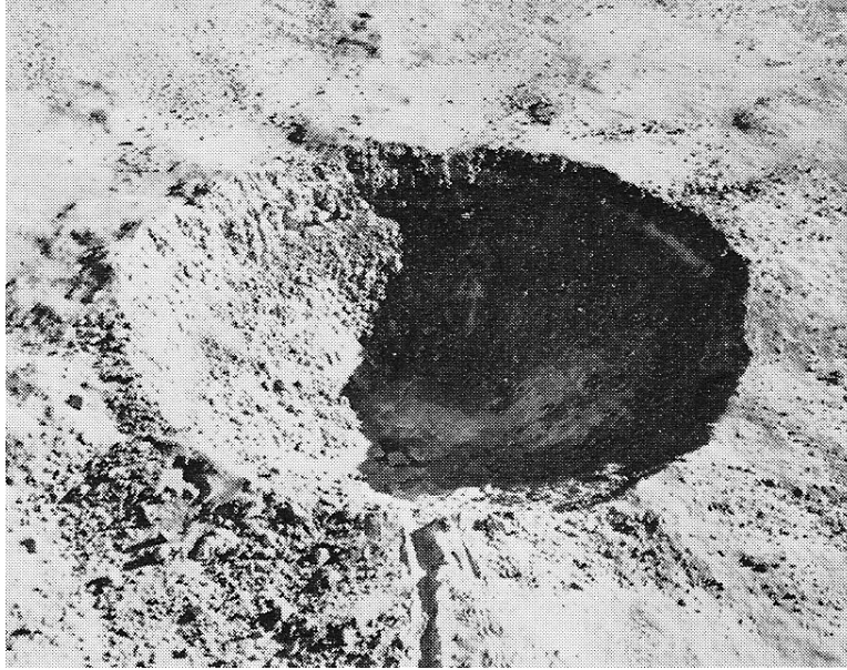
Figure 77. Single cratering 35 kT TNT charge in basalt hard rock, Schooner experiment. Source: LLNL.
