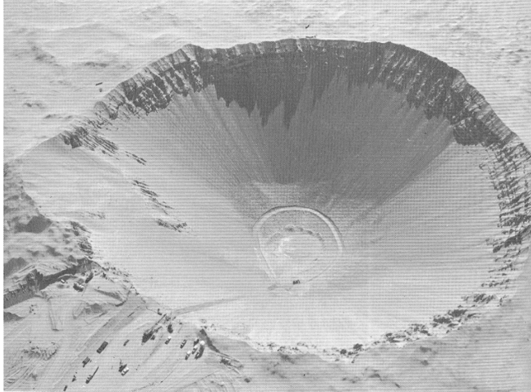
Figure 79. Single cratering experiment in alluvium. Sedan 100 kT TNT experiment. Source: LLNL.
