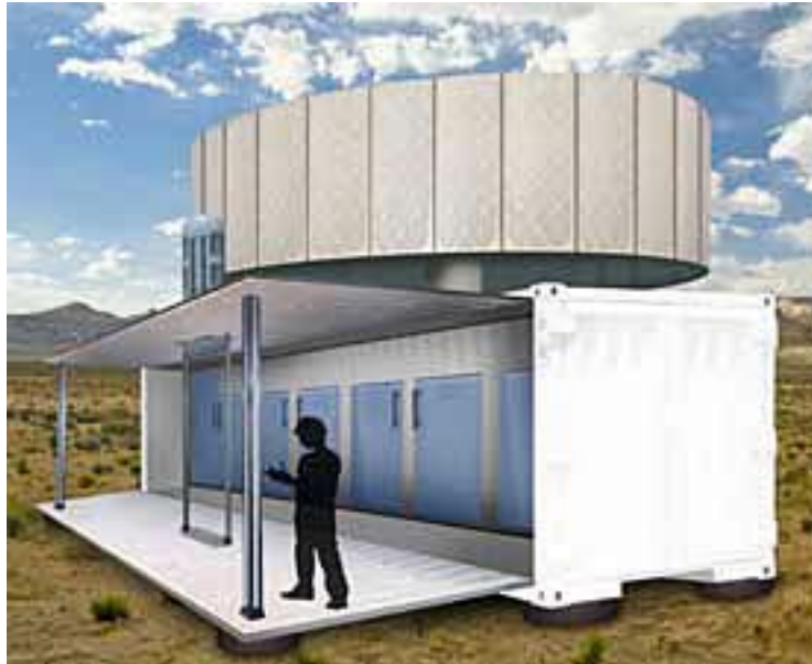
Figure 83. Artificial tree CO 2 catcher conceptual design.
