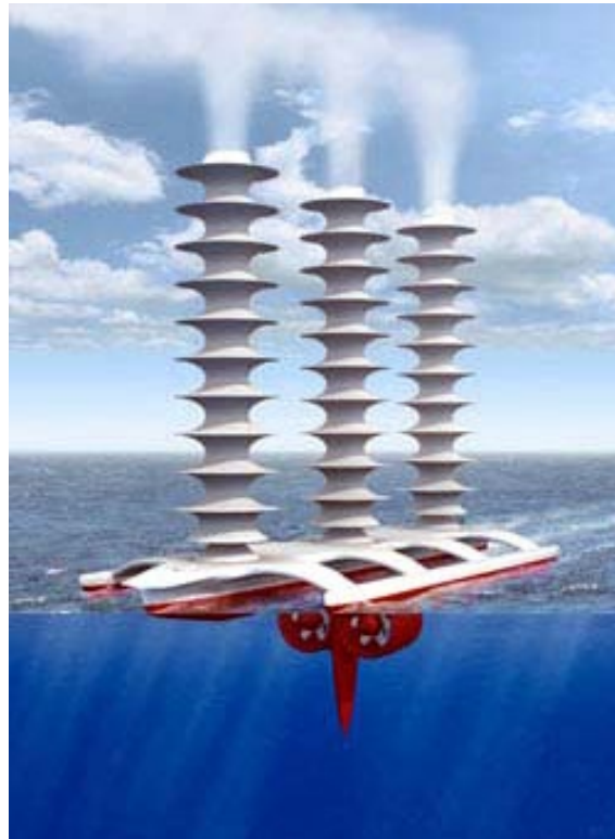
Figure 84. Conceptual designs of cloud seeding towers on ship using Flettner rotors. The rotating towers use the Magnus effect to propel the ship. Source: John McNeil.
