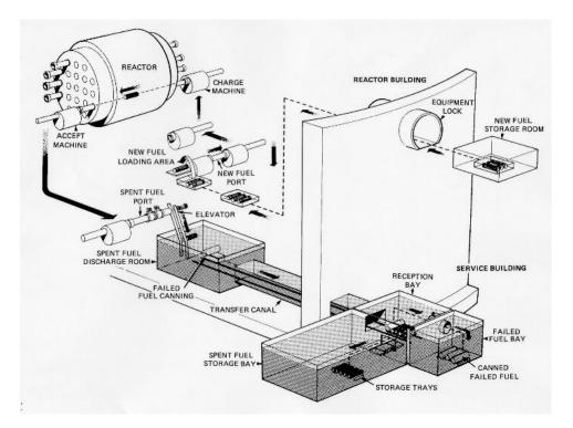
Figure 7. On line refueling machine in horizontal tubes CANDU design.
