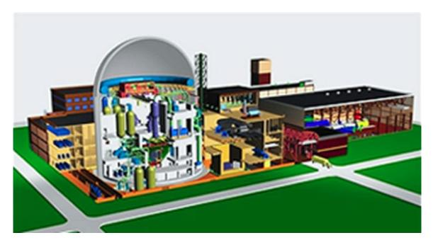
Figure 11. Cutout diagram showing a Candu 9 plant setup.
