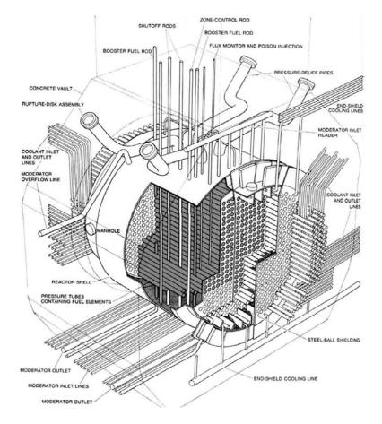
Figure 5. Horizontal calandria of HWR showing its components.
