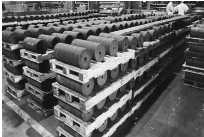
Figure 29. Billets of depleted uranium weighing 1,100 lbs each.
