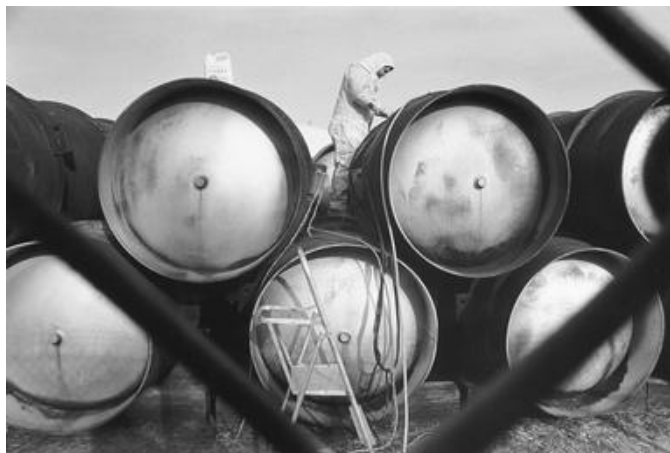
Figure 30. Inspection of UF 6 storage cylinders.
