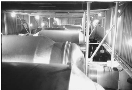
Figure 41. Gaseous diffusion plant cells arrangement showing the compressors and diffusers for the cascade process.
