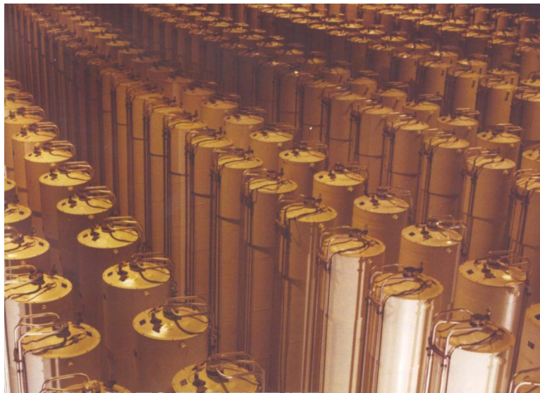
Figure 48. Centrifuge banks at the European Urenco plant (top), and the USA USEC demonstration plant (bottom).
