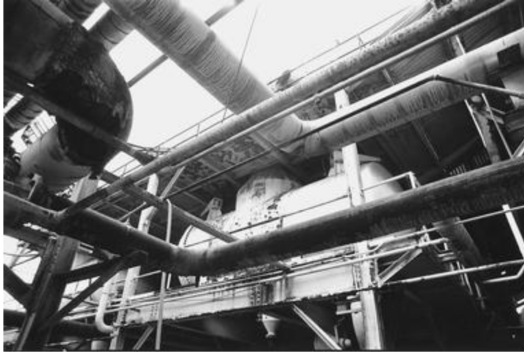
Figure 11. Lithium Column Exchange, COLEX process enrichment equipment. Isotopes of lithium are partially separated when transferring between an aqueous solution of lithium hydroxide and a lithium-mercury amalgam. The isotope \text{Li}^6 has a greater affinity for mercury than does the isotope \text{Li}^7 . A lithium and mercury amalgam is first prepared using natural lithium. The amalgam is then agitated in a natural lithium hydroxide solution. The rare \text{Li}^6 isotope concentrates in the amalgam and the more common \text{Li}^7 isotope migrates to the hydroxide solution. A counter-current flow of amalgam and hydroxide passes through a cascade of stages until the desired enrichment in \text{Li}^6 is reached.
