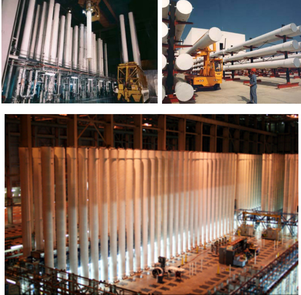
Figure 49. Assembly of third generation Set III centrifuges with annual performance of 200 SWU/yr per machine.
