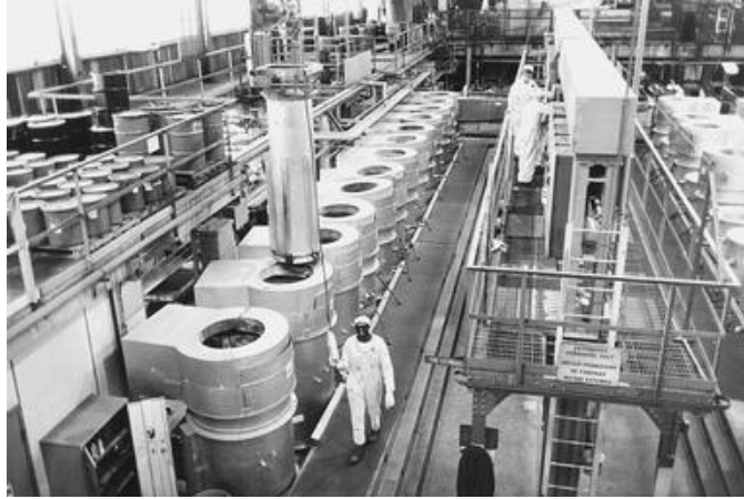
Figure 28. Induction furnaces for the magnesium reduction of uranium metal.
