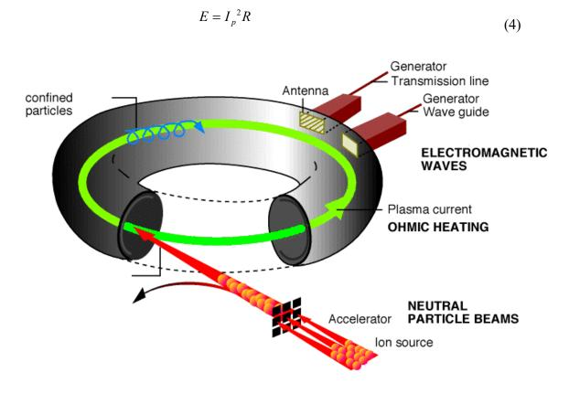
Figure 11. Plasma heating methods.
