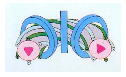
Figure 7. Two possible configurations for the Stellarator coils and magnetic field. In the lower configuration, toroidal coils and helical poloidal coils generate the resulting twisted toroidal magnetic field.
