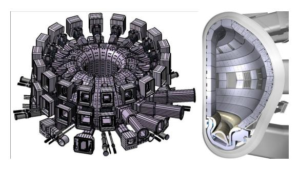
Figure 22. Cross section of the International Thermonuclear Experimental Reactor (ITER).
