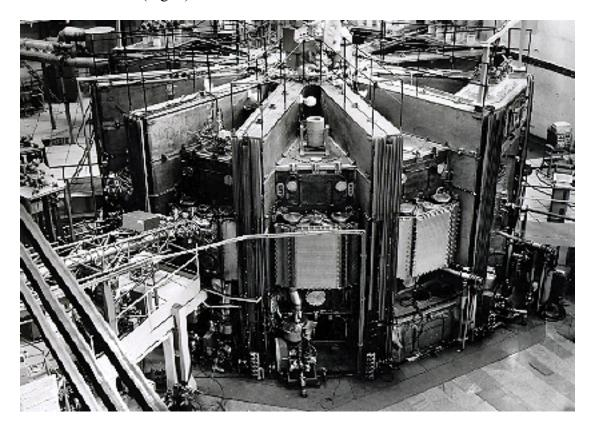
Figure 4. The T-15 Tokamak at the Khurchatov Institute, Moscow, showing its transformer coils.
