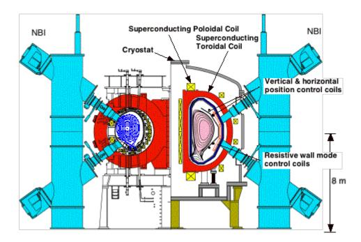
Figure 20. Cross-section of the JT-60 Tokamak.
