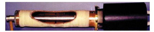
Figure 29. Magnetic flux compression generator. Aluminum tube surrounding a copper wire helix is compressed by a chemical or nuclear explosive. At the other end a transformer couples the generated current pulse to the load. Photo: LANL.
