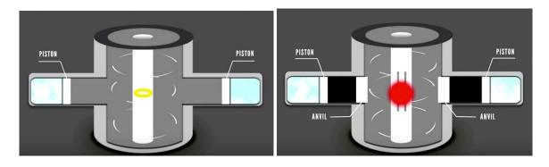
Figure 30. Magnetized target fusion. A plasma is injected into a liquid metal vortex then is compressed by steam-driven pistons.
