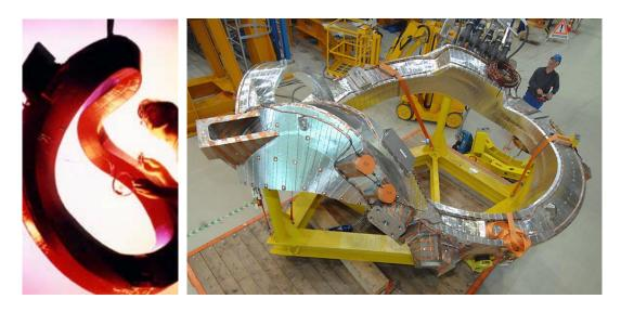
Figure 8. A single superconducting magnet coil for the 7-X Stellarator at Wendelstein, Germany.
