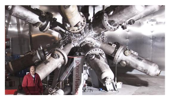
Figure 32. Magnetized target fusion experiment, Vancouver, British Columbia, Canada. Source: General Fusion.
