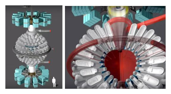
Figure 31. Magnetized target fusion reactor configuration. Liquid metal vortex is surrounded by steam-driven pistons.
