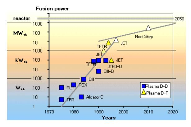
Figure 35. The path towards fusion power production.
