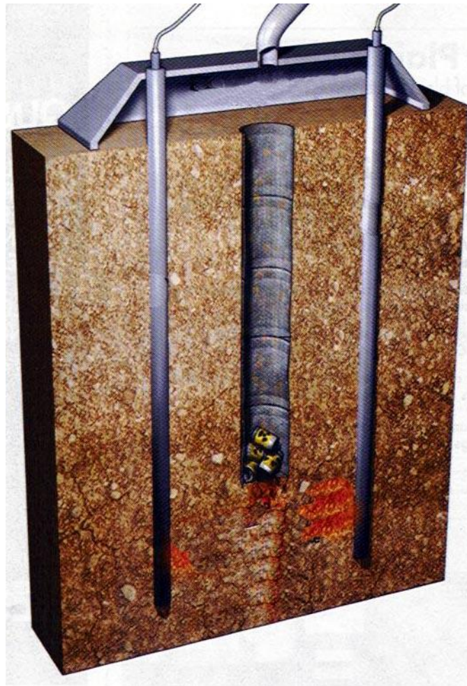
Figure 33. Subsurface vitrification using graphite electrodes.
