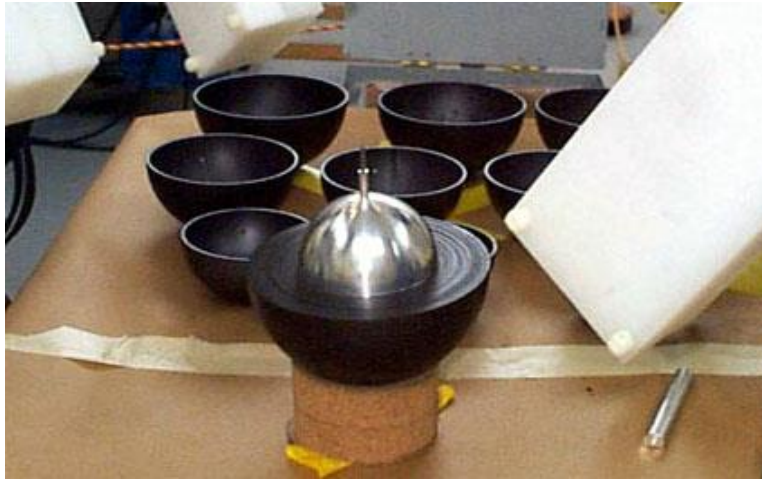
Figure 14. Nickel-clad \text{Np}^{237} in a critical experiment with enriched \text{U}^{235} shells.
