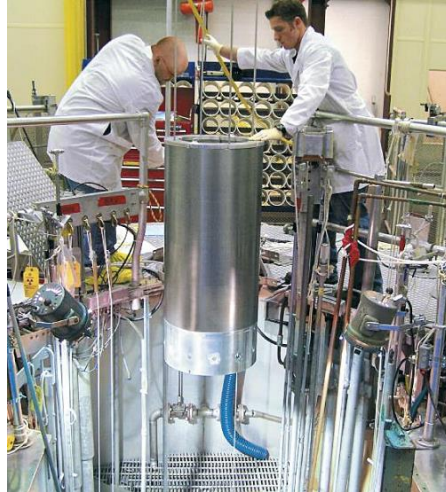
Figure 28. Beryllium neutron reflector being inserted into the University of Missouri Reactor (MURR) for the production of medical isotopes.
