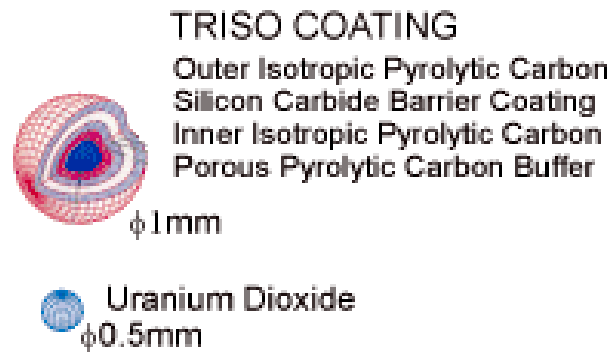
Figure 22. The Triso fuel particles contain 93 percent enriched U 235 or recycled U 233 as fuel in gas cooled reactors. The fuel particle is surrounded by pyrolytic carbon and SiC shells.
