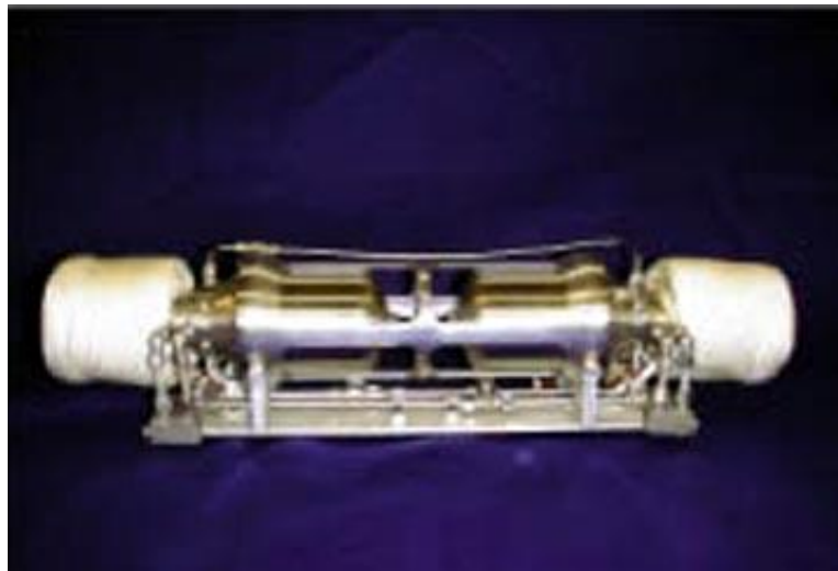
Figure 21. Stirling engine powered by a radio isotope heat source, NASA Glenn Research Center.
