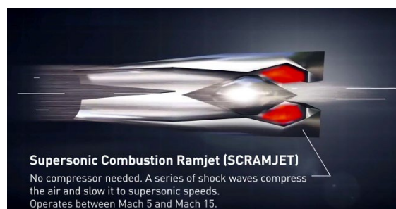
Figure 98. Operation of a ramjet/scramjet engine.
