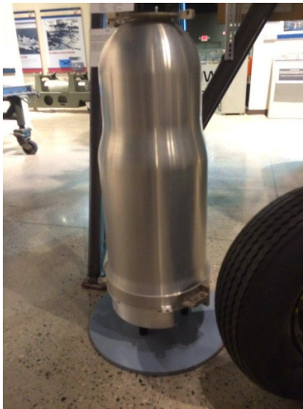
Figure 50. Museum replica of W80 variable 5-170 kT of TNT equivalent thermonuclear warhead.
