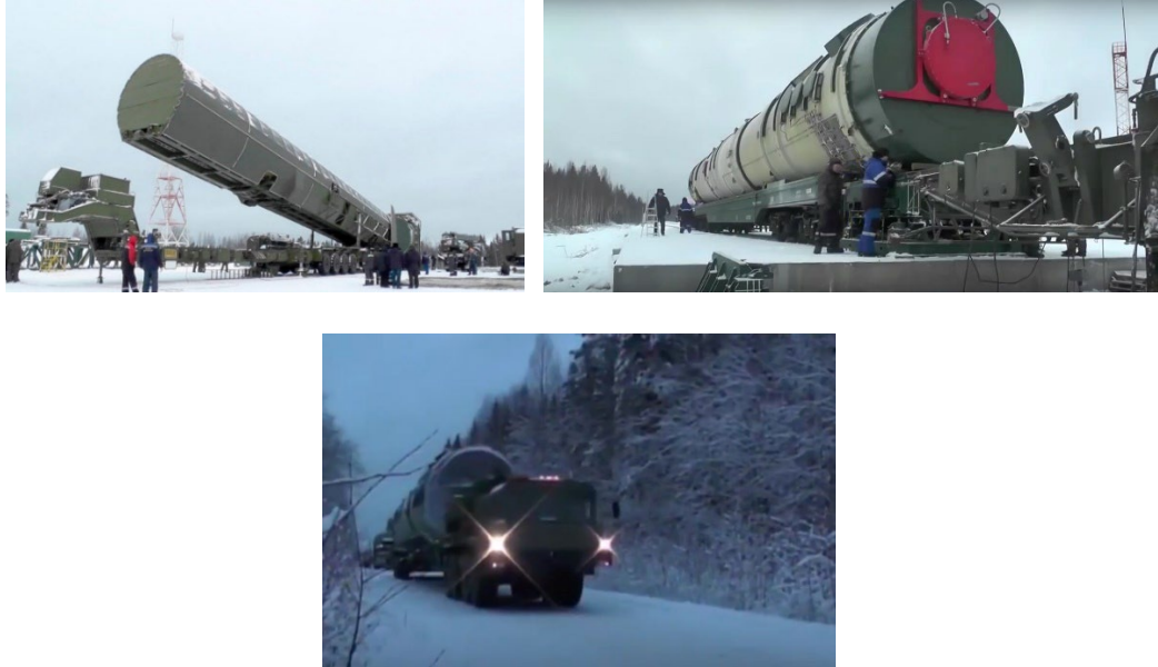
Figure 95. The mobile SARMAT non-ballistic radar evading missile equipped with up to 15 MIRVed reentry vehicles, including decoys.
