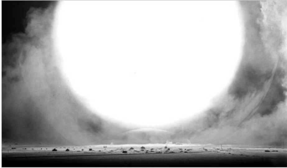
Figure 64. Fireball surrounded by blast wave and its reflection off the ground tested atop military vehicles.
