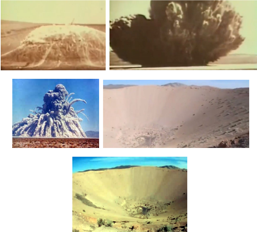
Figure 67. The Sedan underground 105 kT TNT equivalent cratering explosion, July 6, 1962. The release of Cesium 135 and Argon 37 are indicative of underground nuclear explosions.
