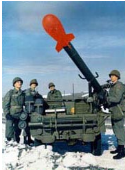
Figure 83. Davy Crockett 20-ton of TNT-equivalent tactical device. The M28 or M29 Davey Crockett weapon system was a tactical battlefield smooth bore recoilless rifle for delivering the W388 nuclear projectile with the W54 nuclear warhead. It was developed during the Cold War. Depending on source its yield was 20 tons of TNT equivalent. It entered service in 1961 and was deployed with USA forces in West Germany.
