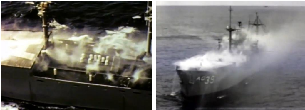
Figure 12. Pressurized sea-water ship decontamination of surviving ships after the Baker underwater test.
