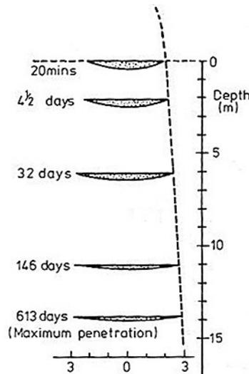
Figure 3. Hypothetical descent of a 3 m<sup>3</sup> lens-shaped immiscible debris pool to a maximum depth 14 m within 613 days.
