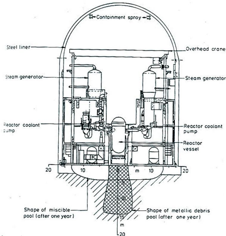
Figure 1. Debris pool for corium penetration of the base mat below a PWR pressure vessel. Miscible pool extent and metallic debris pool shape and depth after 1 year for a hypothetical core meltdown.
