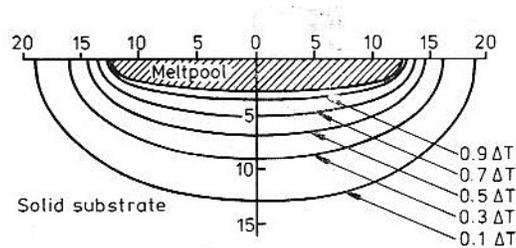
Figure 2. Temperature distribution above the ambient temperature around a miscible pool 13 m in radius and 3 m in depth after 1 year for a 3,000 MWth PWR.
