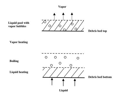
Figure 4. Multilayered once-through debris bed cooling.
