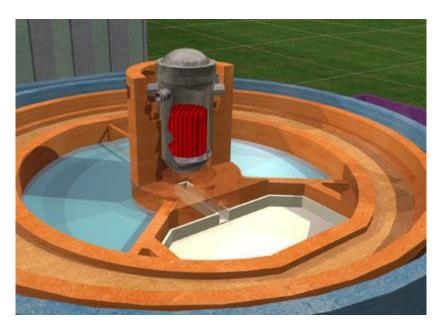
Figure 5. Corium and debris bed cooling system in the Evolutionary PWR, EPWR. Source: Areva.
