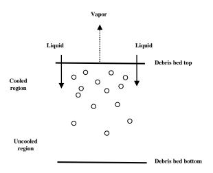
Figure 3. Closed bed debris bed cooling.
