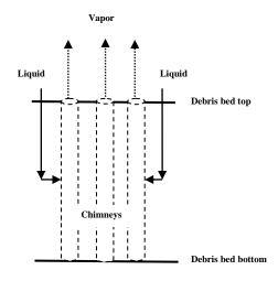
Figure 2. Debris bed chimneys cooling.
