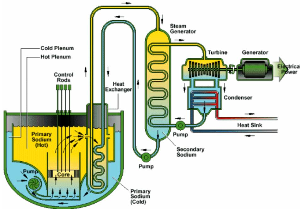
**Fig. 6: The Sodium cooled Fast Reactor (SFR).**
