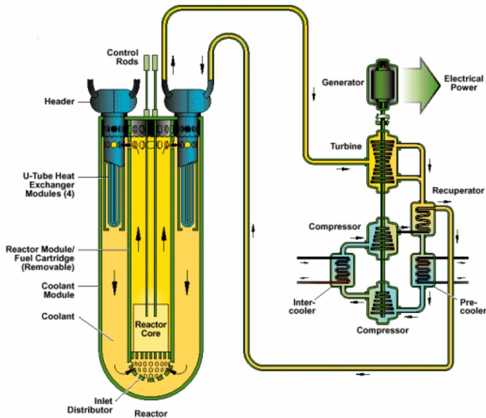
**Fig. 7: Lead cooled Fast Reactor with Brayton, Joule gas turbine cycle.**
