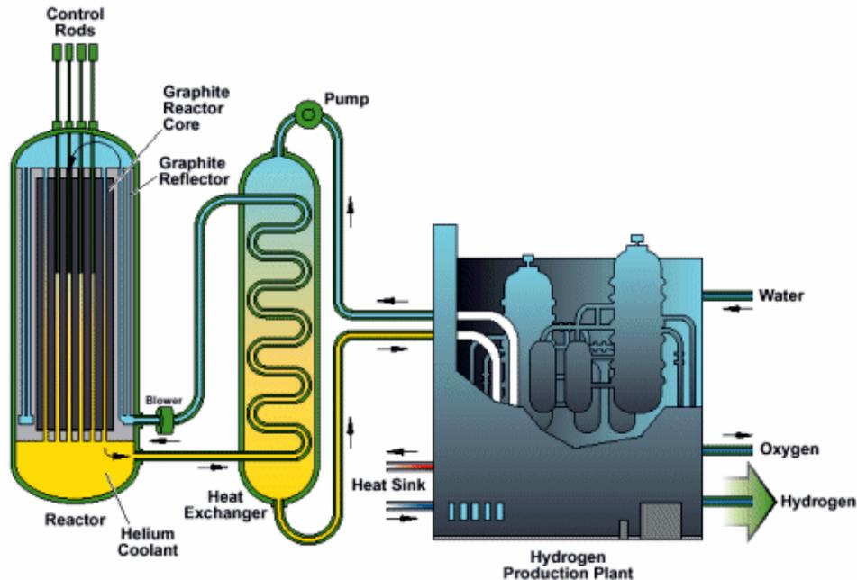
**Fig. 4: Very High Temperature Hydrogen and Electricity (VHTR) design.**
