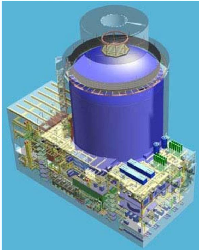
**Fig. 2: Cutout of the AP1000 showing its chimney concrete containment structure surrounding its steel shell containment.**
