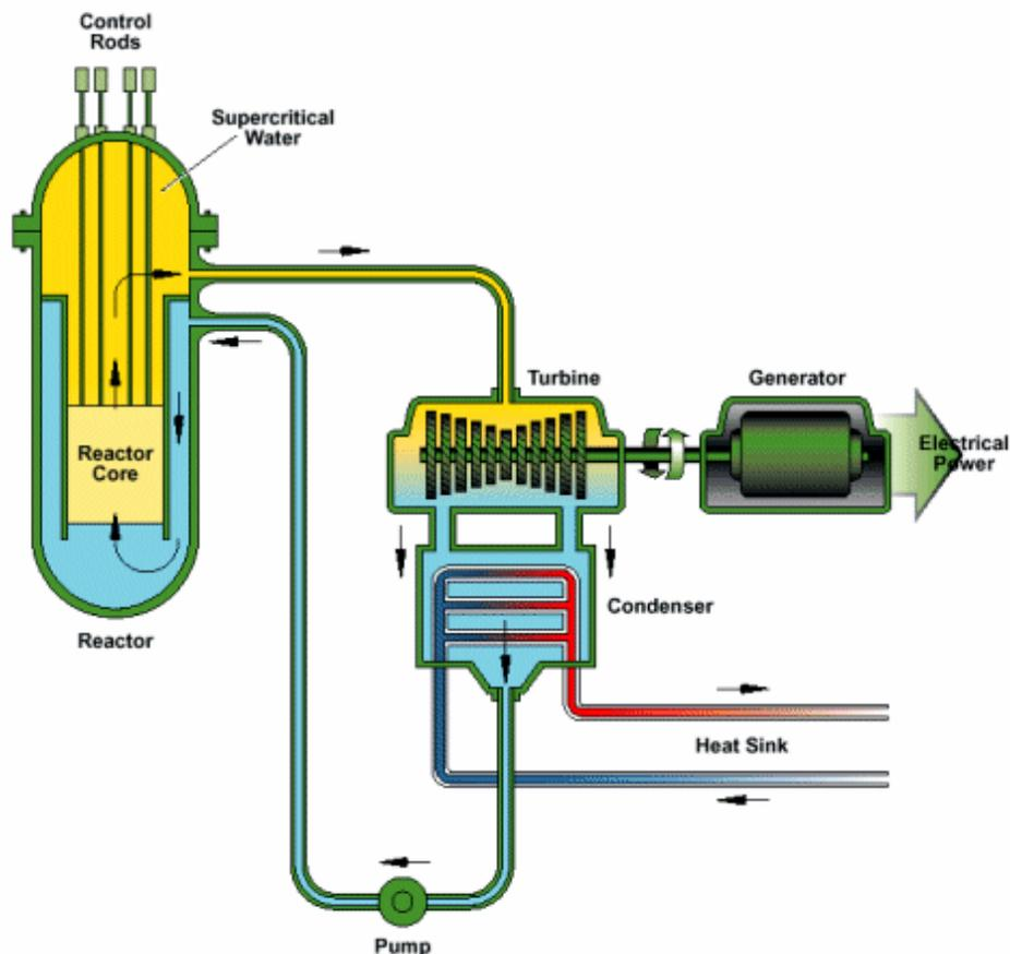
**Fig. 8: Supercritical Water Cooled Reactor (SWCR) using the Rankine steam cycle.**
