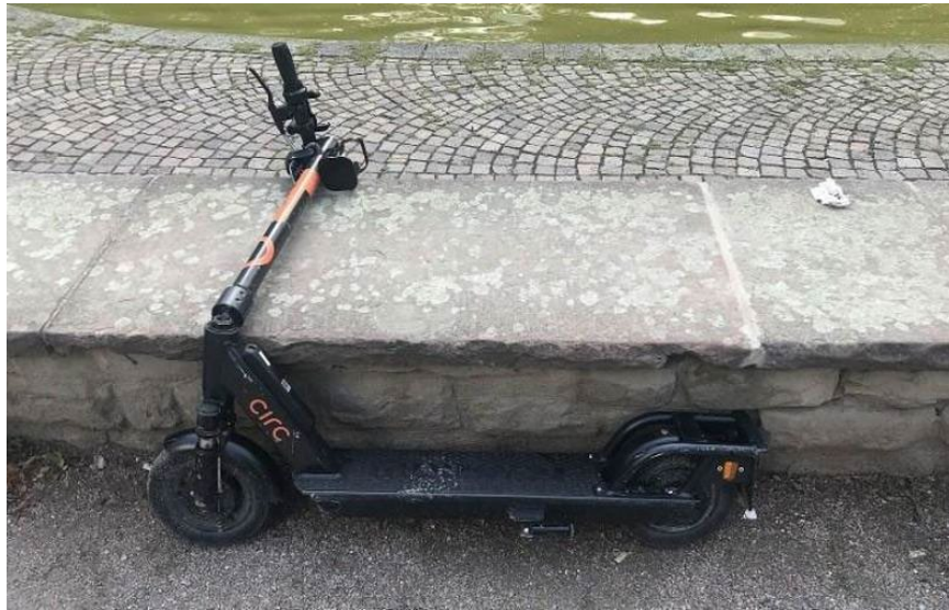
Figure 150. E-scooter broken pole accident.
