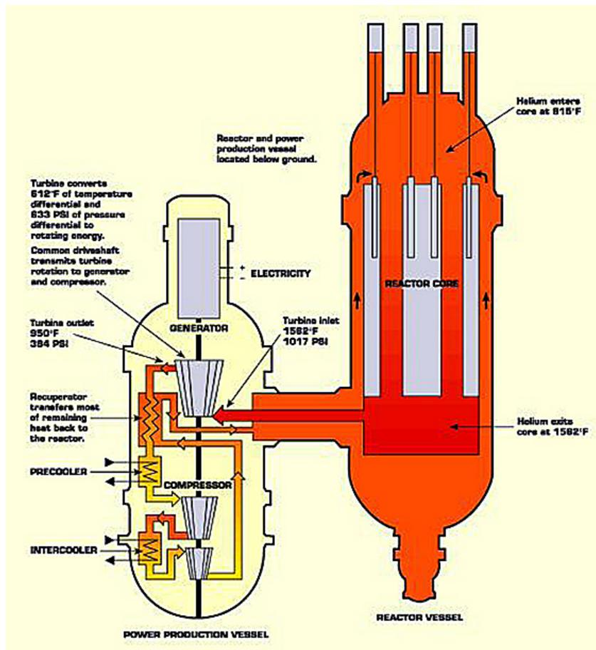
Figure 1. Brayton gas turbine cycle gas cooled reactor configuration.
