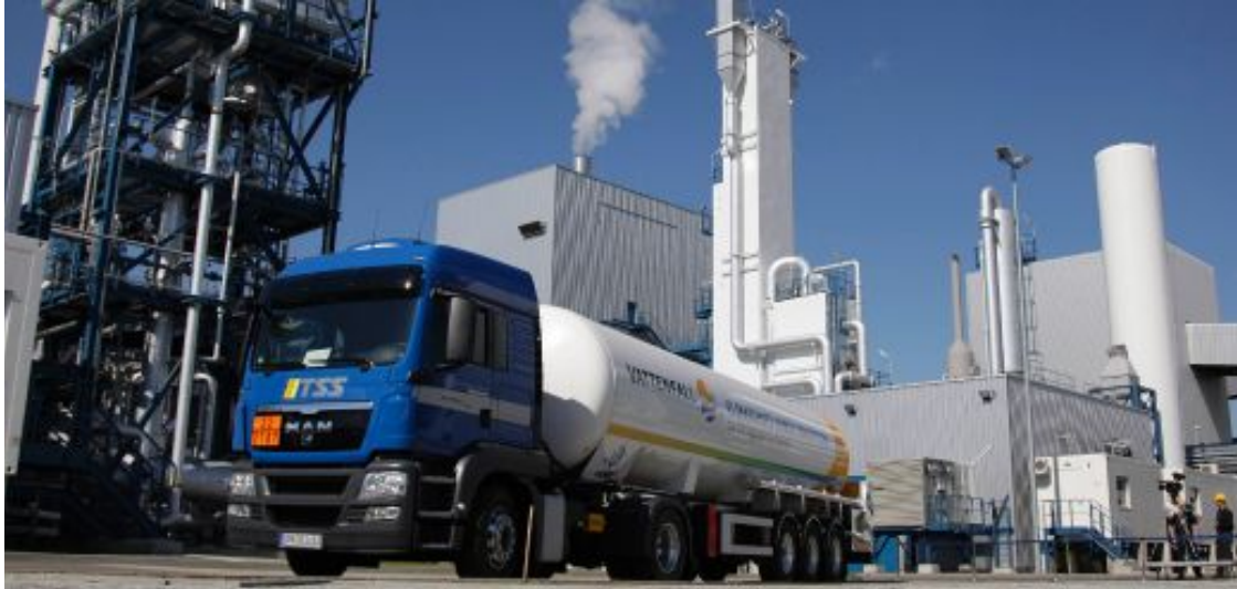
Figure 5. Liquefied CO 2 hauling truck received at the Schwarze Pumpe power plant at Spremberg, Germany, the first plant storing CO 2 deep underground in a saline aquifer. Source: Reuters.
