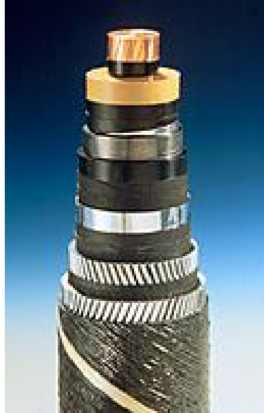
Fig. 5: Layers of a submarine electrical power transmission cable. These cables are mass impregnated (MI) cables suitable for HVDC. The cable has a copper conductor and the insulation is made of oil impregnated paper. There is a lead alloy sheath outside the insulation. Mechanical protection is achieved by steel tape and steel wire armoring. A typical 450 kV HVDC cable has an outer diameter of approx. 13 cm.
