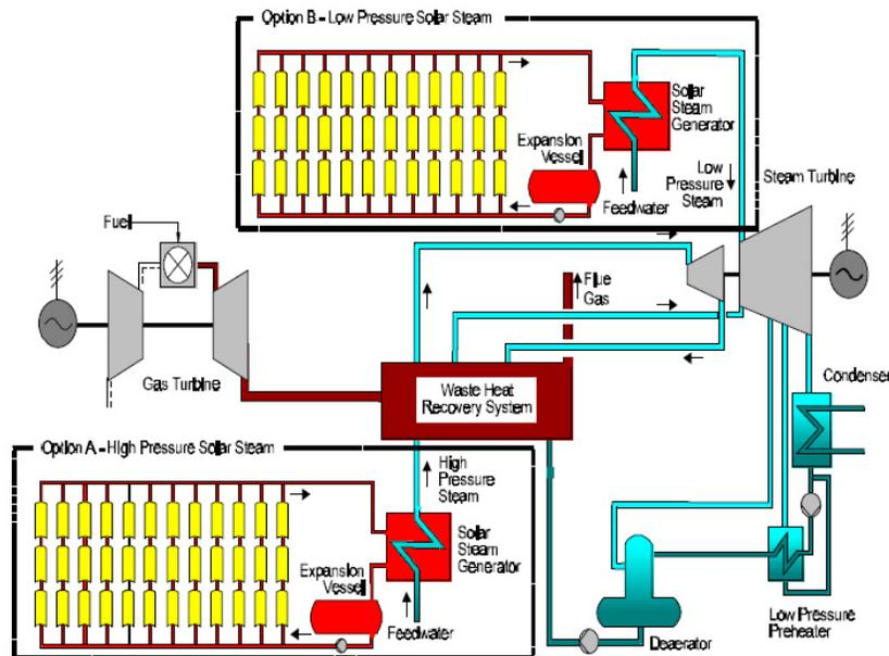
Figure 2. Integrated Solar Combined Cycle, ISCCS thermal system [2].
