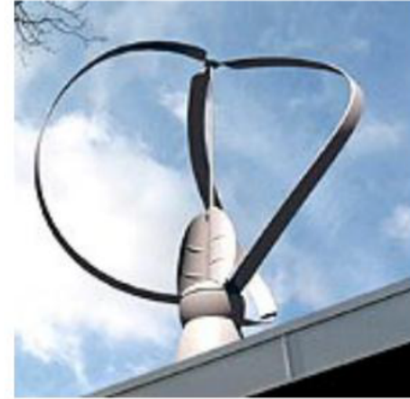
Figure 2. Hybrid Darrieus and Savonius self starting Neoga turbine on top of a building.
