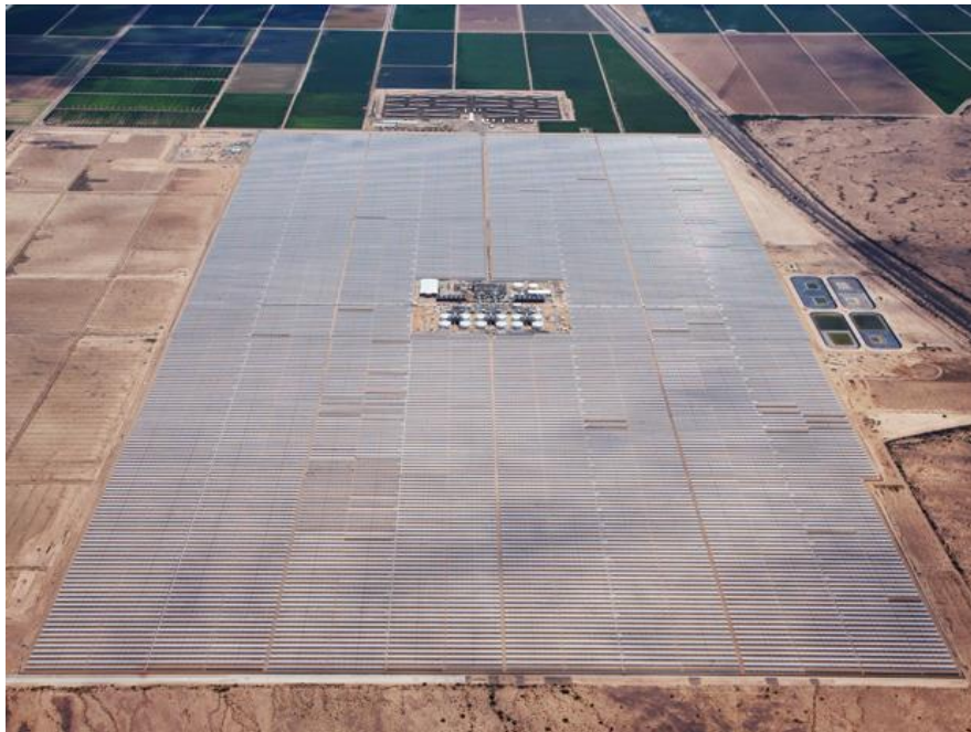
Figure 49. Abengoa Solana 280 MW parabolic trough collector plant at Gila Bend, Mojave Desert, Arizona, uses energy storage in a molten salt.
