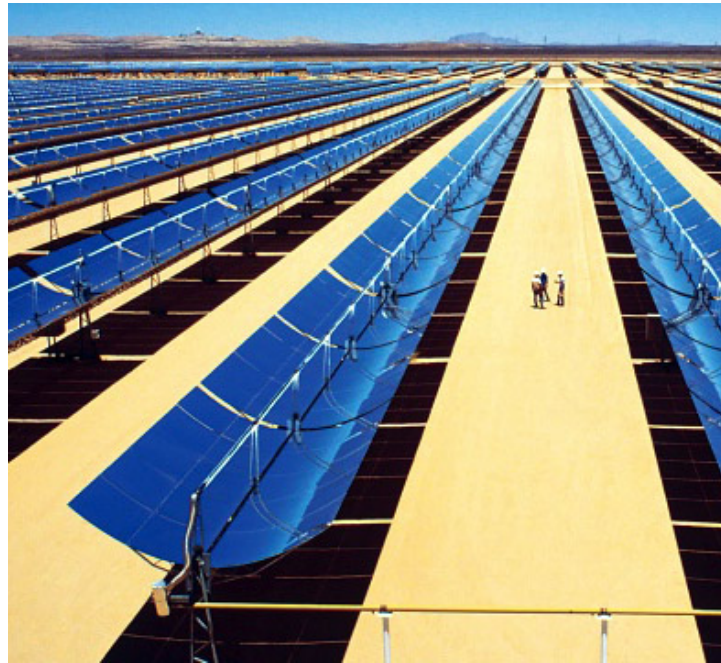
Figure 18. Parabolic trough concentrator using oil as a working medium at 752 oF or 400 oC. Kramer Junction, California, USA. Source: Der Spiegel.
