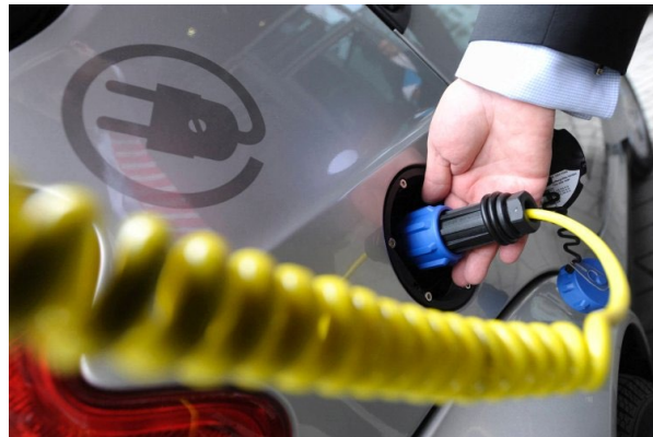
Figure 20. Plug-in electric cars could charge their batteries overnight with electricity supplied by electrical power plants. Norway with large hydroelectric power resources is planning a primarily electric transportation fleet. A battery-equipped car fleet would effectively act as a distributed energy storage system.
