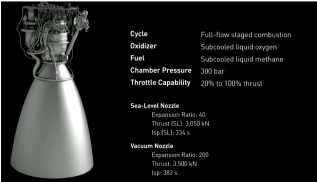
Figure 40. Raptor engine design. Specific impulse of 334-382 is predicted. Source: Space X.
