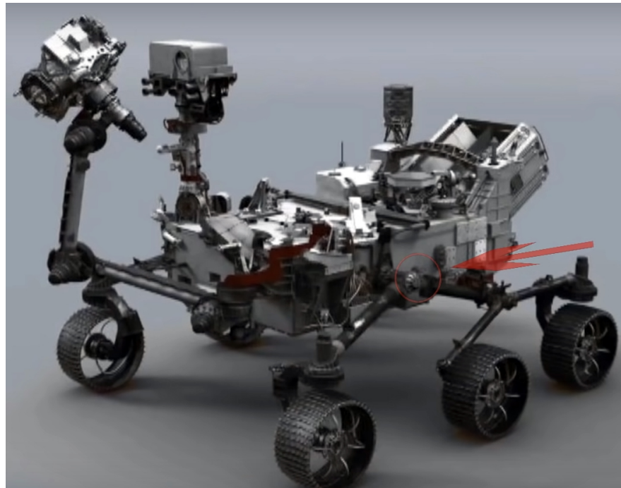
Figure 26. Mars Perseverance Rover. Will extract oxygen from the Mars' atmosphere as fuel for future retrieval missions. Source: NASA.
