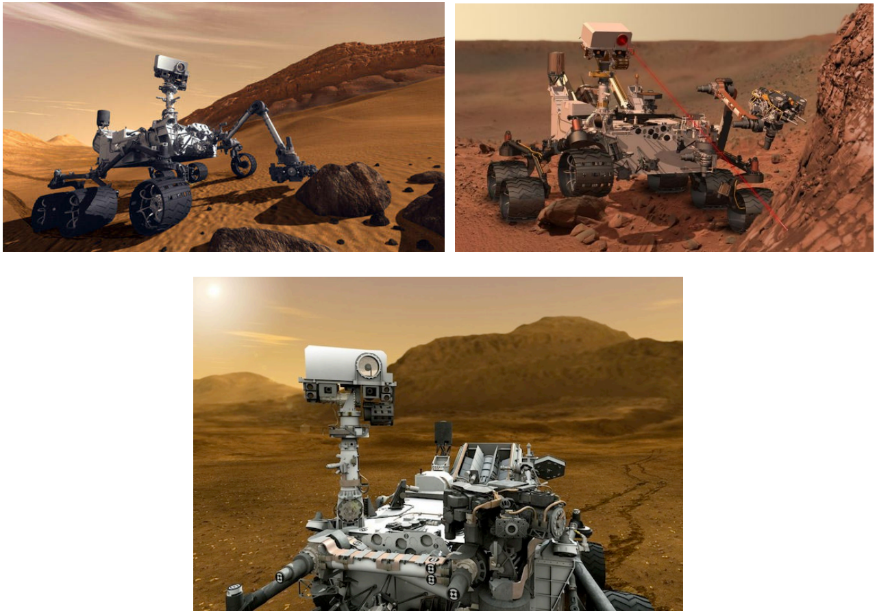
Figure 25. Mars Science Laboratory mission Curiosity rover uses its Chemistry and Camera, Chem Cam, instrument to investigate the composition of a rock surface. It fires infrared laser pulses at a target and views the resulting spark with a telescope and spectrometers to identify chemical elements. Source: NASA.
