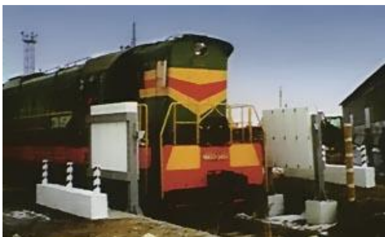
Figure 44. Nuclear materials radiation detector proportional counters portal system for trains.
