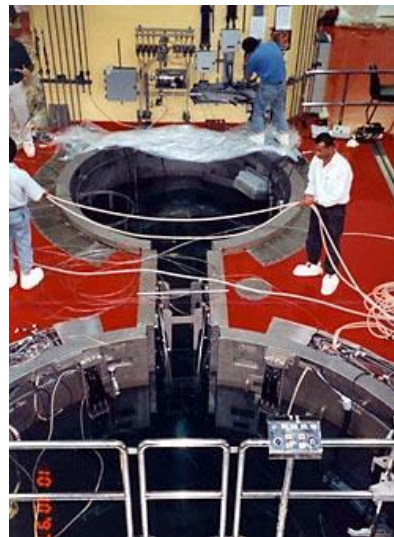
Figure 19. Interior views of the ETRR-2, open pool type 22 MWth research reactor at Inshass, Egypt.
