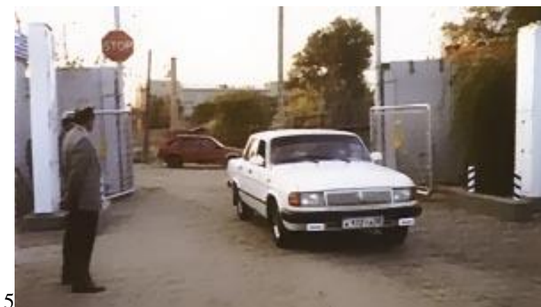
Figure 43. Nuclear materials proportional counter monitors for pedestrians and cars at Astrakhan on the Caspian Sea.
