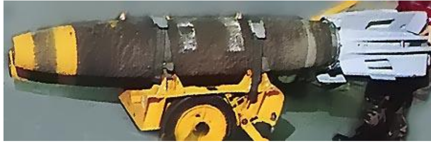
Figure 55. Five hundred pounds Joint Direct Attack Munition (JDAM) on its cart, showing the directional steering and control fins.
