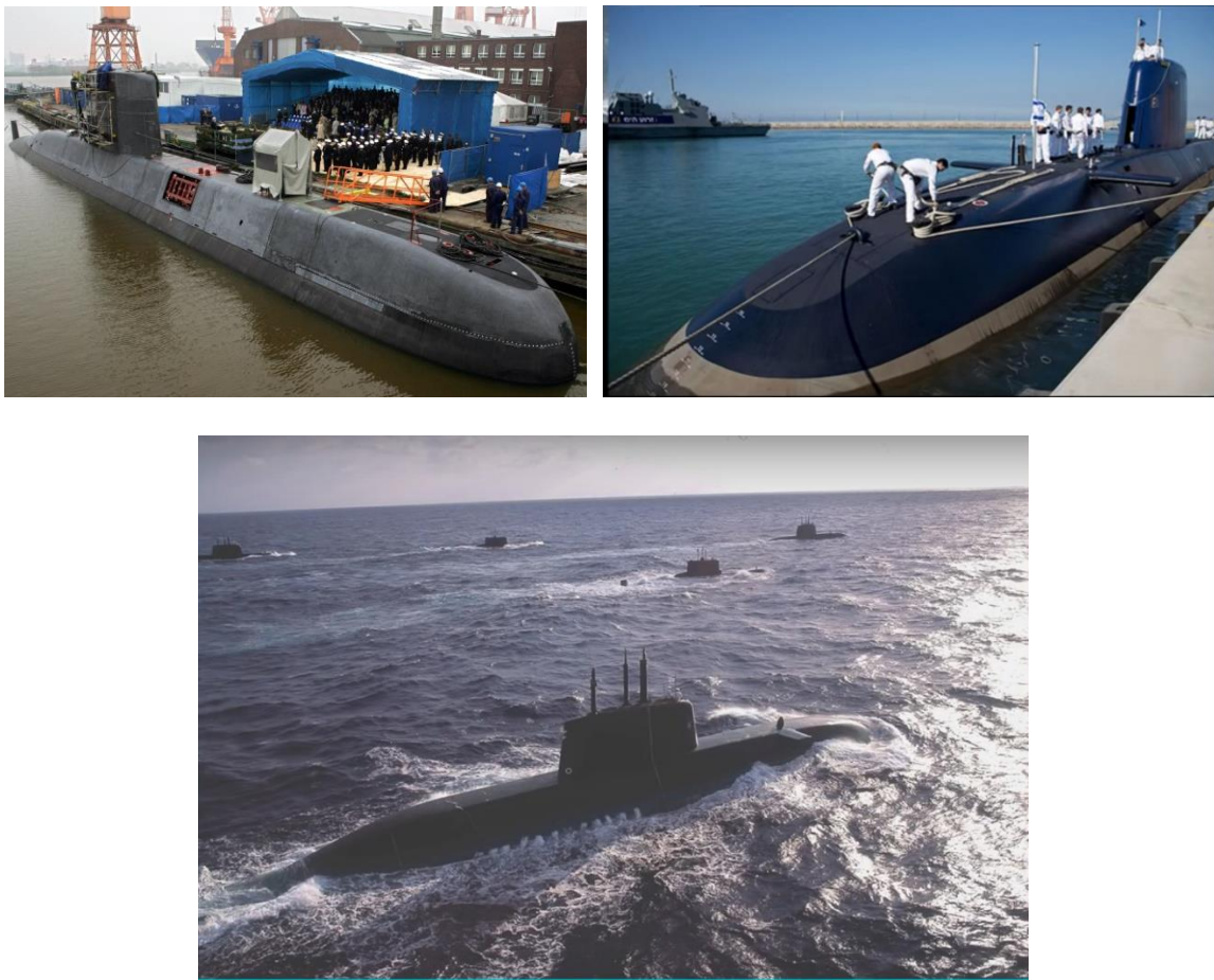
Figure 33. The exclusively-for-export Type 209/1400 class German attack submarine delivered to South Africa, 2005, is not operated by the German Navy (top left). The 3-5 Dolphin class submarines used by the Israeli Navy are based on the Type 209, but are highly modified and enlarged. Flotilla of 5 fuel-cell submarines reportedly armed with nuclear tipped cruise missiles (top right, bottom).
