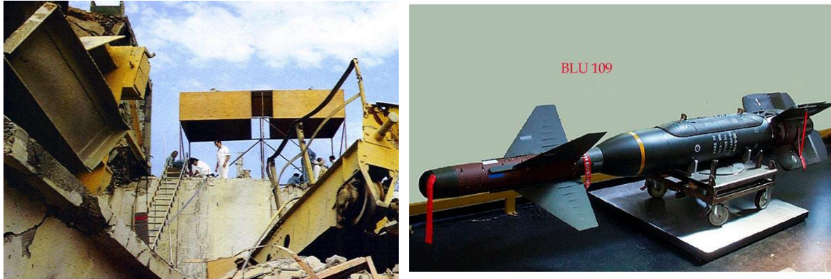
Figure 12. Testing dispersed fuel at a bombed-out, using BLU-109 penetrator bunker buster munitions by the USA, Tuwaitha research reactor in the 1991 Gulf War. Picture is a variant of a Guided Bomb Unit GBU-24( )/B. The warhead is a BLU-109( )/B penetrator (warhead = Bomb, Live Unit ), and the guidance/tail kit is from the Paveway III family. Together, it is called a GBU-24/B. If a Joint Direct Munition (JDAM) guidance system kit is strapped on it, it would be a GBU-31.
