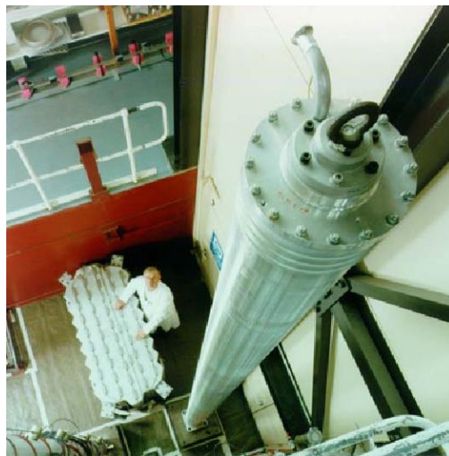
Figure 22. European-design Urenco single gas centrifuge.
