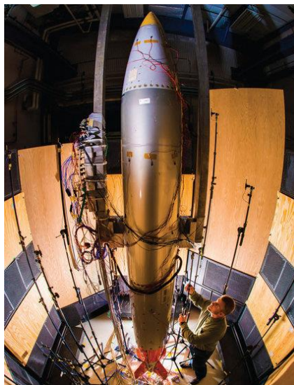
Figure 72. The B61 Model 12, small-yield, stealth and precise nuclear munition. It has a "dial-a-yield" feature whose lowest setting is only 2 percent as powerful as the bomb dropped on Hiroshima in 1945. Source: Sandia Laboratory.
