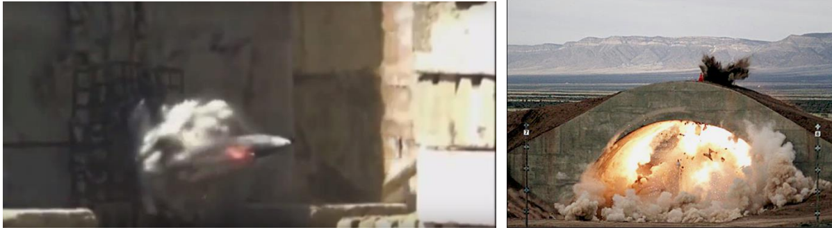
Figure 62. Earth penetrator bunker buster munition consists of a shaped charge front component followed by a hardened case penetrator.
