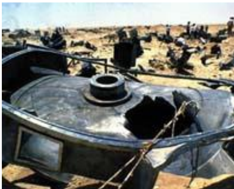
Figure 14. Destroyed vacuum chamber casing of a single experimental Calutron electromagnetic separation device.
