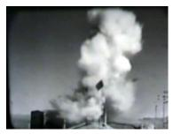
Figure 2. Progression of the Borax experiment into a steam explosion in a BWR. Notice the falling debris. Video grabs.
